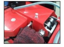
• Adjust the depth stop and tighten the counter nut to fix it well.
