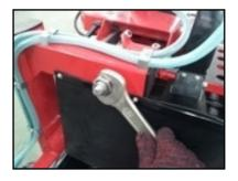
• Rotate the cutting head until it stops at 45°.
