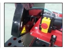
Loose the left threaded hexagonal nut on the motor shaft and remove the outer flange and the tool.
