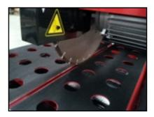
Put the material on the cutting table. By using the back square control the position of the material.
