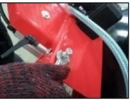
Make sure that the blade is not touching the cutting table at any position of the table when the cutting head is at the lowest position.
