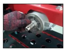
• Mount the new blade. Make sure the tool rotation is correct and the bore corresponds to the shaft diameter.
