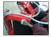
Rotate the cutting head until it stops at 0°.
