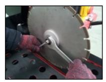
• Close the blade guard. Tighten the screw at the front and on the side.
