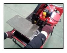
Push the cutting table slowly and without undue pressure towards the rotating blade.
