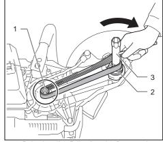
1. Pulley (small) 2. Pulley (large) 3. Box wrench
