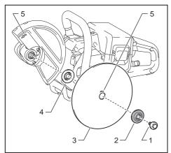
1. Hex bolt 2. Outer flange (black) 3. Abrasive cutoff wheel / diamond wheel 4. Inner flange (silver)
