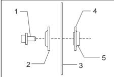
Hex bolt 2. Outer flange (black) 3. Abrasive cutoff wheel / diamond wheel 4. Inner flange (silver)
