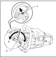
1. Shaft lock button 2. Box wrench 3. Tighten
