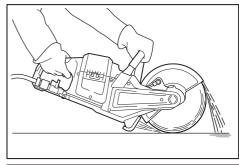
**NOTE:** When the battery cartridge temperature is low, the tool may not work to its full capacity. At this time, for example, use the tool for a light-duty cut for a while until the battery cartridge warms up as high as room temperature. Then, the tool can work to its full capacity.
