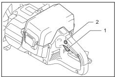
1. Switch trigger 2. Lock-off button
