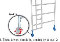
These towers should be erected by at least 2 competent persons. Apply brakes and fit adjustable castors into one 4 rung ladder frame and one 4 rung main frame,ensuring that spring loaded pin is engaged in hole provided (see detail 1A).
