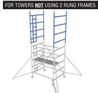
5. Working from platform add a 4 rung ladder frame to the 5 rung ladder frame by locating onto head fitting with peg engaging into hole provided. Repeat the process at the other end using a 4 rung main frame.
