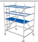
3. Fit 2 long braces diagonally in opposite directions as close to the vertical tube as possible. Fit a temporary platform on the 3rd rung down from the top of the frame &, working through the trap fit short braces as temporary guardrails horizontally onto top & 2nd rung of frames between pegs provided. Level the tower by adjusting collar on castors (see construction notes)
