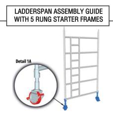
1. These towers should be built by at least 2 competent persons. Check you have the correct equipment & it is in working order. Apply brakes & fit adjustable castors into both 5 rung frames ensuring that spring loaded pin is engaged in hole provided (see detail 1A).
